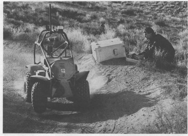
TEARING AROUND THE TRACK — SARGE was shipped to the Army/Marine Joint Programs Office in 1995, but engineer Bryan Pletta (5516) still uses its predecessor, Dixie, to run tests on the Robotic Vehicle Range track southeast of Area 1. Six years of experience with Dixie led designers to create a more adaptable, more capable robot with SARGE. (Photo by Randy Montoya)
